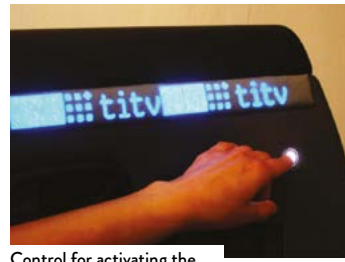
Control for activating the lighting in spacer fabrics integrated in door paneling
