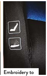
Embroidery to display a stored control unit for adjusting the seat position
